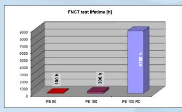
Minimum service lives in the FNCT "Full Notch Creep Test" according DVS 2205-1 supplement 6.
